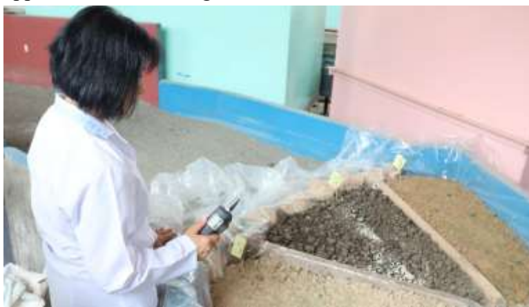
Fig. 1 Experimental setup for comparative assessment of water percolation through PMM-modified and control mine-tailings substrates
